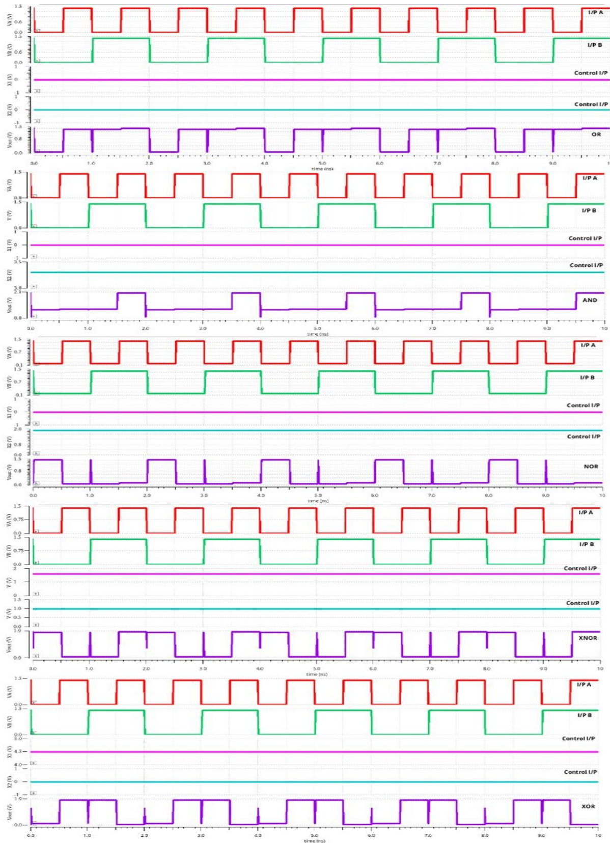
Fig. 10. Transient simulation for 2-operands QGSFET for different control voltages.
