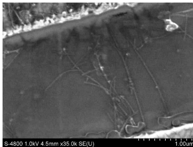
Fig. 1. FESEM image of aligned SWCNTs bridged across Au electrodes. The increased diameter (~45 nm) indicates non-covalent functionalization with Fe(II)Pc.
